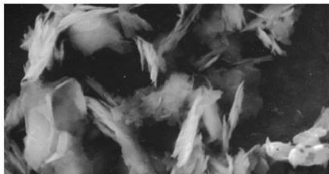
SEM image of Mistron® Vapor @ 2000 magnification
